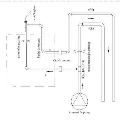
Picture 4.5 Piping installation principle diagram
