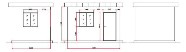
Picture 4.1 Color steel plate monitoring station recommended size map
