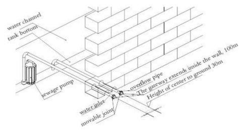
Picture 4.4 Schematic diagram of pipe installation
